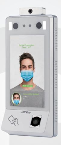
G4[TD] is a fully upgraded version of the G4 Visible Light Facial Recognition Terminal using intelligent engineering facial recognition algorithms and the latest computer vision technology. It supports speedy facial recognition with large capacity and other authentication methods, including identification with fingerprint, card, and password. G4[TD] also enhances security performance in all aspects.
