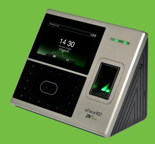
uFace800 facial multi-biometric time & attendance and access control terminal supports up to 3,000 face templates, 4,000 fingerprint templates and 10,000 cards.
