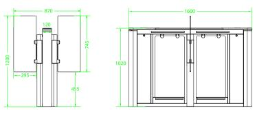
\* Turnstile can work in the temperature of -20°C to 70°C. If the temperature is under -20°C, acrylic parts may be broken. (Temperature control device is optional to solve this problem.)
