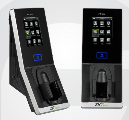
**inPulse** is an IP-based finger vein access control terminal that works as a standalone device or connected to a third party access control panel using Wiegand interface. With patented vein recognition technology, inPulse is able to identify fake or dry fingers, and providing excellent performance under strong sunlight.
